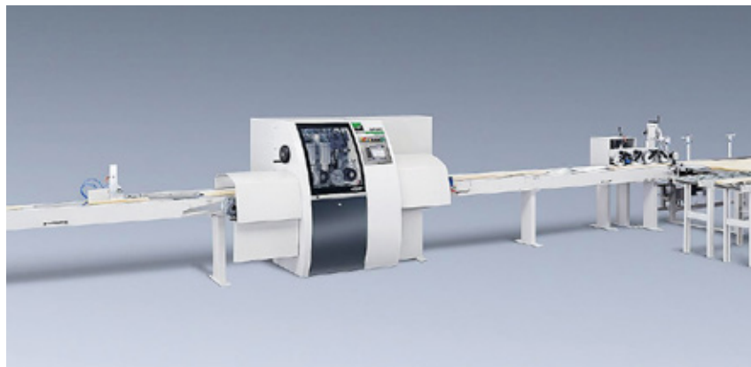
Weinig Dimter's high-performance cross-cut machines, like the OptiCut 450 Quantum, cut out defects. Then, the workpieces enter ...
